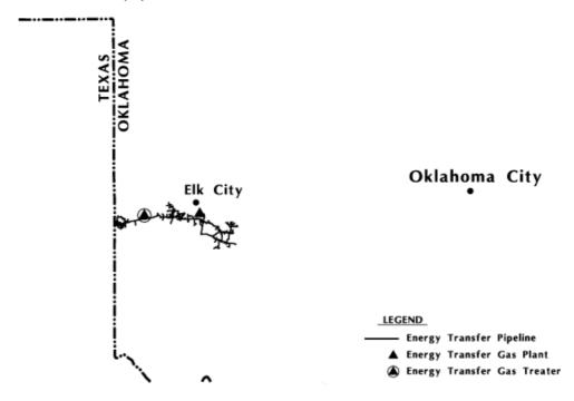
General. The Elk City System is located in western Oklahoma and consists of over 315 miles of natural gas gathering pipelines, the Elk City processing plant and the Prentiss treating facility. The gathering system has a capacity of approximately 410 MMcf/d and average throughput was approximately 170 MMcf/d for the 11 months ended August 31, 2003. There are five compressor stations located within the system, comprised of 18 units with an aggregate of approximately 19,000 horsepower.
